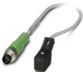
Sensor/actuator cable, 2-position, PUR, gray RAL 7001, Plug straight M8, on Valve connector Festo KMYZ9, with 1 LED, cable length: 0.3 m
